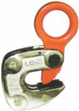
④ Horizontal Clamp Rated load: 1T/2T/3T Clamping range (mm) 1-13/3-22/12-35
