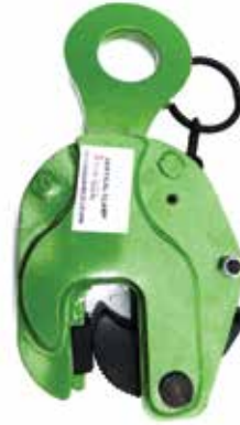
⑥ Vertical Clamp Rated load: 1T/2T/3T/5T/7T/10T Jaw Opening (mm) 0-20/0-30/0-35/0-45/0-50/0-50
